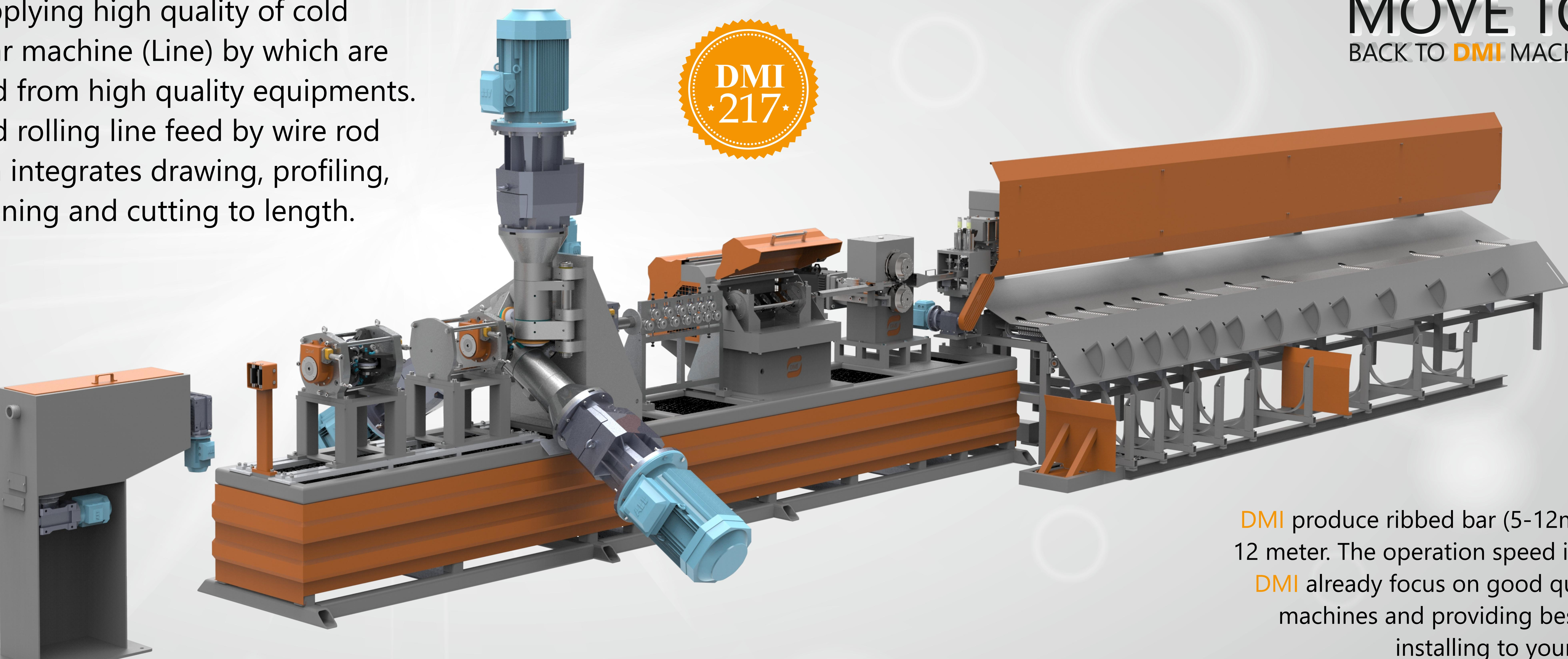
DMI produce ribbed bar (5-12mm) with max. length 12 meter. The operation speed is max. 300 m/minute.
